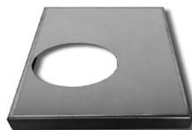
Another element supplied in gas-fired ovens is the flame guard, also in stainless steel, which must be positioned above the flame output of the gas burner and will protect the oven's cooking chamber from the direct flame, deviating it on the vault in order to distribute and uniform the heat over the entire surface of the chamber.
